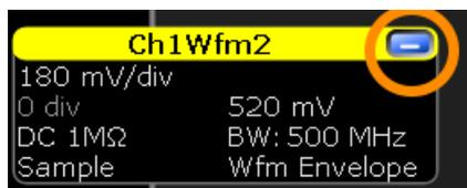
The diagram is removed and the signal icon on the sidebar displays a live view of the signal.
