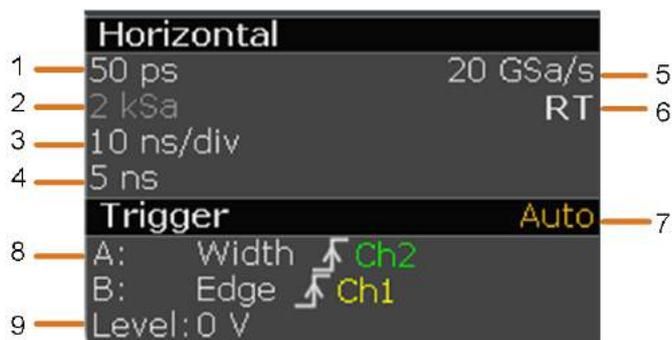
**Figure 7-2: Horizontal and trigger label on top of the sidebar**
